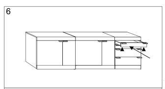
Place the drawers in the body. To do this, pull the drawer runners out, place the drawers on them and slide them back in. If necessary, the height of the drawers can be adjusted by means of the wheels underneath the drawer.
