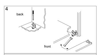
Level the bodies by turning the adjustable legs and the adjusting brace (only in combiantion with a separation) which are under the bottom, with a spanner. Then mount the plinth and place the cap cover (C).
