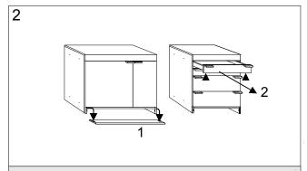
First demount the plinth (1) and then, if present, the drawers. To do this, grip the snappers on the underside of the drawer, and pull forward.
