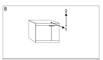
When replacing the top: first slide the top to the front and then lift it.
